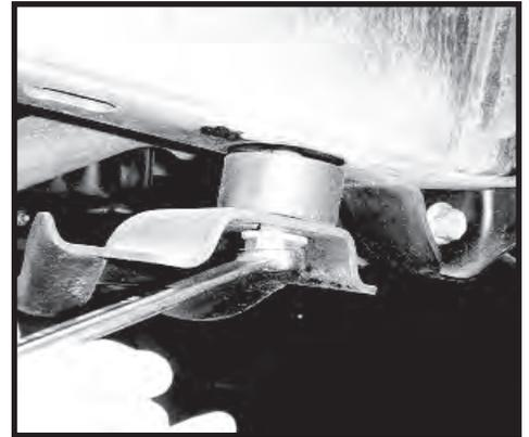
Step 1. Remove the factory engine skid plate (if equipped). Do not discard hardware it will be re-used later.
