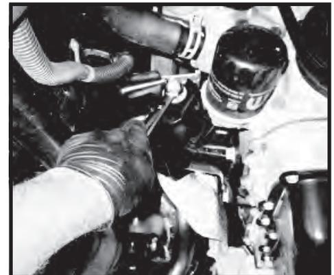
Step 4. Place the driver side skid plate mount onto the engine frame mount. The large slotted opening goes on the main engine bolt. When installing the bracket feed the M10 bolt thru the bottom hole in the skid plate bracket. Place a washer and nylock nut onto the bolt. Do not tighten at this time. Repeat for other side.
